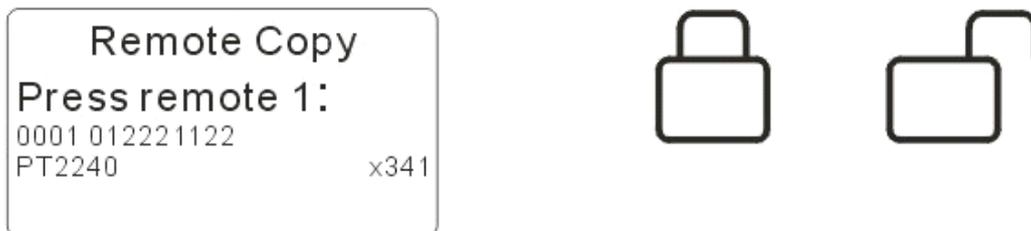
If the data is suppose to be incorrect, please press the button again until you think it's correct. Then short press "Enter", the screen will display "Press remote 2". Keeping the remote always on "Induction zone" and press the next button you want to copy, other buttons and so forth.
