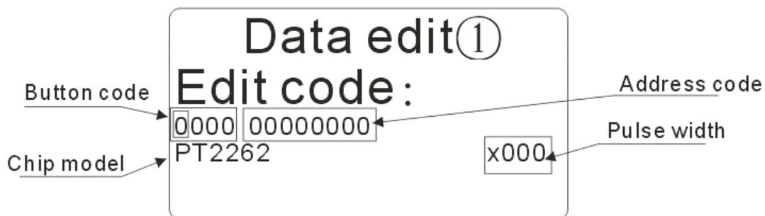
**Edit button code:** For fixed code, different chip have different number of buttons. For example, LX918 only have 3 buttons, but PT2262 have 4. In our Host, two separately area stands for button code and address code. The 3 or 4 numbers on the left stands for button code, the right one after the blank stands for address code.
